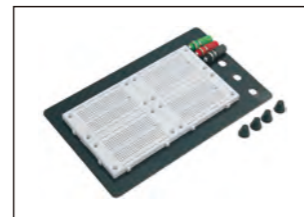
ITEM:EB06B-4S 1080 tie-point 8 Power lanes,160 PTS 4 Standard double-strips,920 PTS SIZE: 16.7×9.1×0.83 cm
