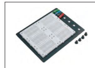
ITEM:EB06B-6S 1620 tie-point 12 Power lanes,240 PTS 6 Standard double-strips,1380 PTS SIZE:16.7×13.65×0.83 cm
